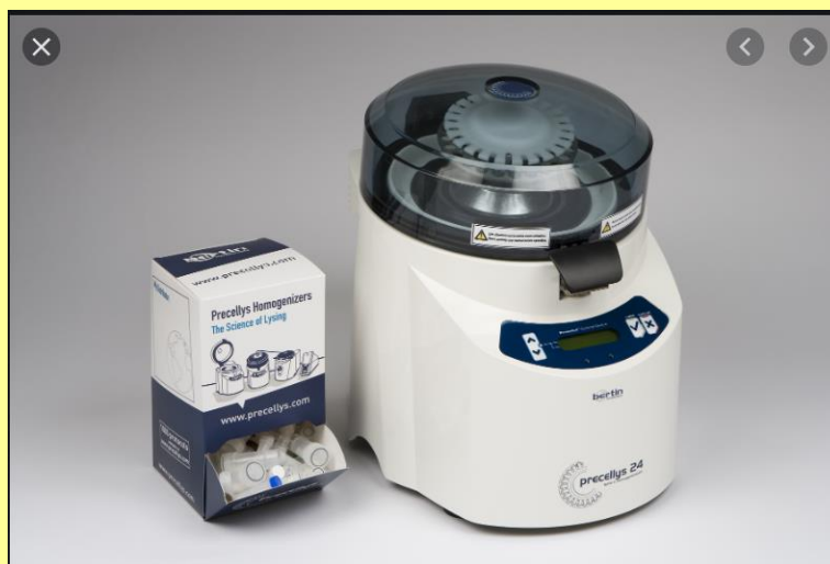
Precellys Homogenizer for pulverization of hair samples
